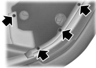
2. From underneath the vehicle, partially remove the tire splash shield by removing four drive screws from the lower flap.
