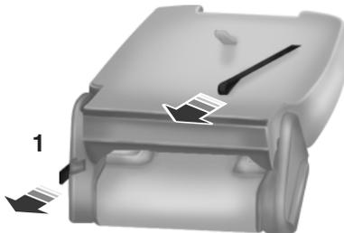
2. To return the seat back to the upright position, pull the number 1 strap. Then, while holding the number 1 strap, pull the long strap located on the seat back to raise the seat back.
