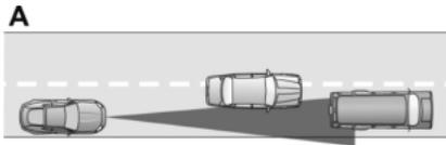
A. When driving on a different line than the vehicle in front.
