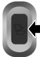
Press the control located at the back of the rear door opening one time to fold the seat back down. Tumble the seat forward for access to the third row.
