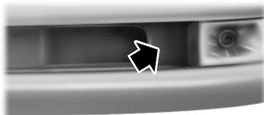
A message regarding a blocked sensor is displayed if the radar signals from the sensor have been obstructed. The sensor is located behind a fascia cover near the driver side of the lower grille. A vehicle ahead cannot be detected and the system will not function when the
