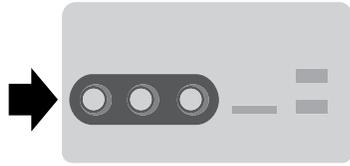
Your A/V inputs allow you to connect an auxiliary audio/video source (such as a gaming systems or a personal camcorder) by connecting RCA cords (not included) to these input jacks. The jacks are yellow, red and white and are located either behind a small access door on the instrument panel or in your center console.
