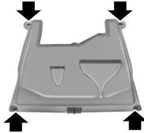
Some vehicles may be equipped with an aero-shield under the engine. This shield needs to be removed for service, including oil and filter changes. It is secured with four quick release fasteners.
