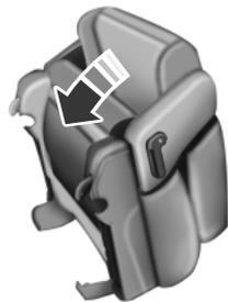
2. To return the seat back to the floor from tumbled position, rotate the seat down until you hear it latching to the floor.
