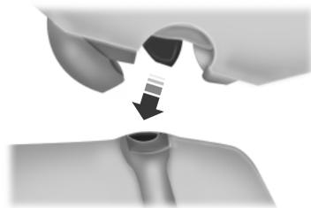
4. Make sure that the rear latch hooks are properly engaged with the floor striker.
