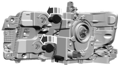
3. Remove the bulb socket by turning it counterclockwise and pulling it straight out.
