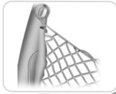
The cargo net secures lightweight objects in the cargo area. Attach the net to the anchors provided. Do not put more than 50 pounds (22 kilograms) in the net.
