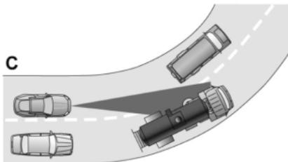
C. There may be issues with the detection of vehicles in front when driving into and coming out of a bend or curve in the road.
