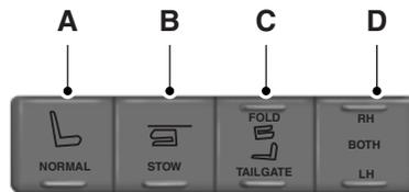
Press the seat selection button (D) to select either right-hand seat, the left-hand seat or both. First, select the seat you would like to adjust, then select one of the following:
