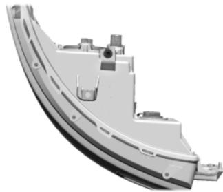
4. Locate the vertical adjuster on each headlamp. Using a Phillips #2 screwdriver, turn the adjuster either clockwise or counterclockwise in order to adjust the vertical aim of the headlamp. The horizontal edge of the brighter light should touch the horizontal reference line.
