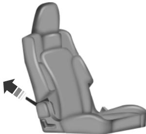
1. Pull the strap located on the back of the second row seat. This will fold the seat back forward. Pull the strap a second time to tumble the seat forward, allowing easy exit from the third row seat.
