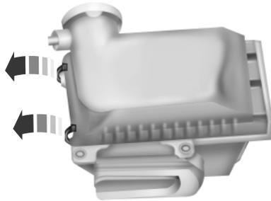
1. On the passenger's side of the air filter housing, release the two clamps from the air filter housing cover.
