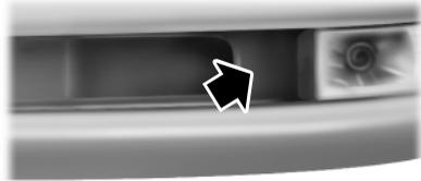
If a message regarding a blocked sensor appears in the information display, the radar signals from the sensor have been obstructed. The sensors are located behind a fascia cover near the driver side of the lower grille. When the sensors are obstructed, a vehicle ahead cannot
