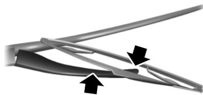
1. Grab the wiper arm with one hand close to the arm/blade joint and pull it as far away from the glass as possible. Do not use excessive force because it can break the wiper arm at the heel. Hold it there until the next step.
