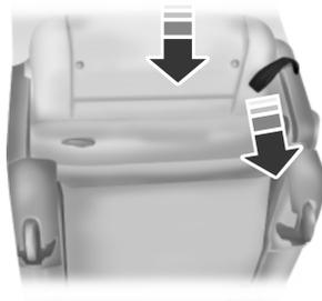
3. To return the seat back to the floor from tumbled position, rotate the seat down until you hear it latching to the floor.
