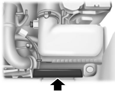
3. Remove the bolt cover (if equipped).
