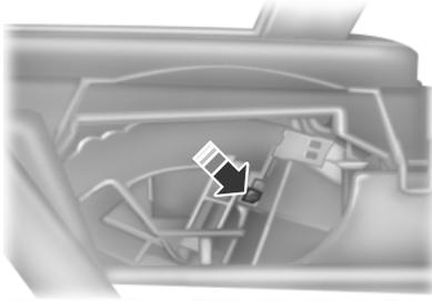
4. Locate the brake shift interlock lever on the passenger side of the shifter assembly.
