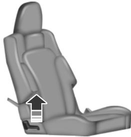
1. Lift the handle located on the side of the seat.
