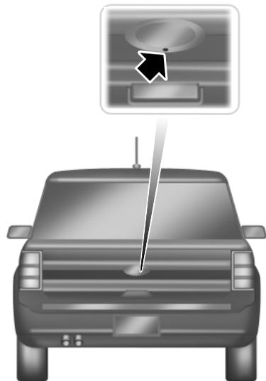
The rear view camera system provides a video image of the area behind the vehicle.
