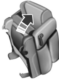
2. Lift the handle all the way up until the seat releases from the floor. Rotate the seat forward, grabbing the bottom of the seat back as indicated, to allow access to the third row seat.
