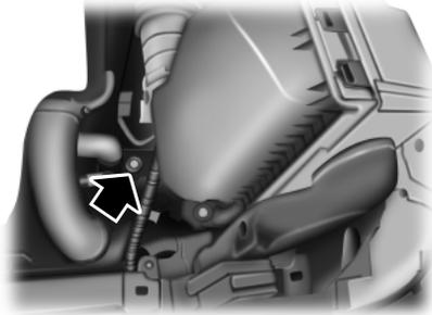
8. Rotate the air filter assembly 90 degrees counterclockwise and reinstall into the rubber hose.
