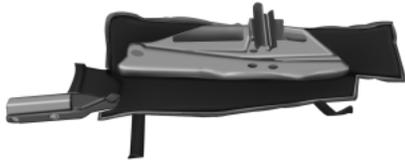
1. Fully collapse the jack, fold the lug wrench socket into the handle and place the jack and wrench into the felt bag as shown. Place the extension bolt or L-shaped bolt into the external pocket of the felt bag. Take care to position the jack as shown to make sure that the locating holes in the jack base can be placed on the locating tabs of the jack mounting bracket in the spare tire tub.
