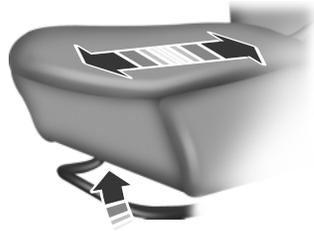
Lift the control to adjust the seat forward or backward.
