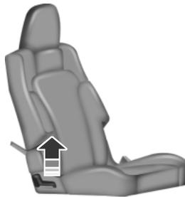
Lift the handle to adjust the seat back rearward or forward. You can also fold the seat back forward until it is flat.
