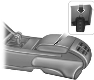
1. Locate the key backup slot in center console utility compartment.
