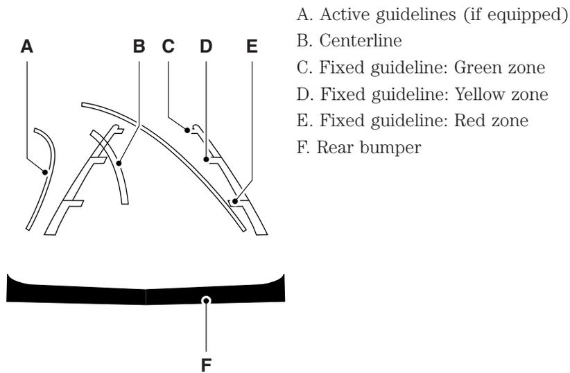
If your vehicle is equipped with active guidelines they are only shown with fixed guidelines. To use active guidelines, turn the steering wheel to point the guidelines toward an intended path. If the steering wheel position is changed while reversing, the vehicle might deviate from the original intended path.
