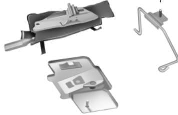
6. Remove the jack, L-shaped bolt, and the wrench from the felt bag. Fold down the wrench socket to use to loosen the lug nuts and to operate the jack.
