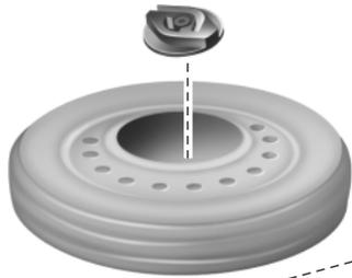
3. Remove the carpeted floor panel located in the rear of the vehicle, then remove the wing nut that secures the spare tire by turning it counterclockwise.
