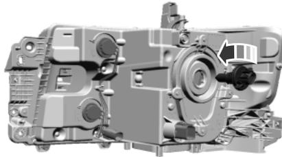
4. Remove the bulb socket by turning it counterclockwise and pulling it straight out.
