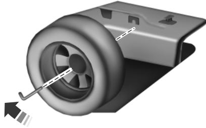
If you are stowing the flat tire, remove the L-shaped bolt from the external pocket of the felt bag. With the third row seat in the raised position, stand the flat tire in the rear of the vehicle with the tire's valve stem facing the rear of the vehicle. Fasten the flat tire to the vehicle by inserting the L-shaped bolt through one of the lug bolt holes in the wheel. Turn it clockwise into the threaded hole in
