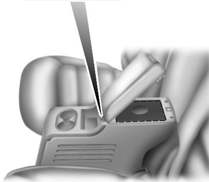
**Refrigerator:** Briefly press and hold **COOL**. The indicator light on the cool side of the switch will illuminate and the indicator light on the freeze side will glow when the refrigerator is active. The temperature will cool to approximately 41°F (5°C). Briefly press and hold **COOL** again to turn off the refrigerator. Briefly press and hold **FREEZE** to change to freezer mode.
