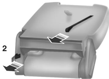
3. Release the cushion latches by pulling the number 2 strap while pulling on the strap located at the top of the seat back. This will tumble the seat all the way into the floor tub.
