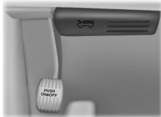
1. Inside the vehicle, pull the hood release handle located under the bottom of the instrument panel near the steering column.
