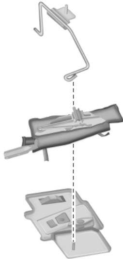
4. Insert the straight end of the jack retention bracket through the eyelet of the angled bracket and swing the retention bracket over the jack. With the jack in place, place the looped end of the retention bracket over the threaded stud in the trunk floor and secure it with the plastic wing nut.
