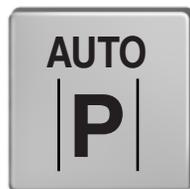
Press the button; the touch screen displays a message and a corresponding graphic to indicate it's searching for a parking space. Use the turn signal to indicate which side of the vehicle you want the system to search on.
