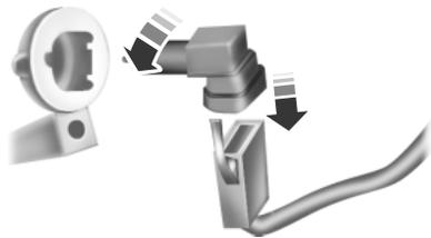
3. Carefully disconnect the wire harness connector from the bulb by releasing the two snap clips.
