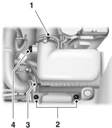
2. Clean the area around the clamp that connects the air filter assembly to the rubber hose (1).
