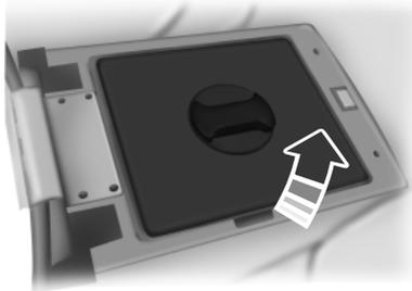
Flip the console lid forward, then lift off the cover to open the cooling compartment. Make sure to replace the cover after you using it. This helps maintain a more consistent cooling temperature.
