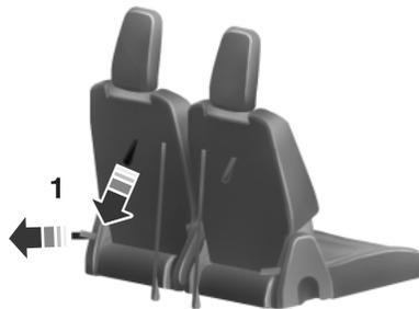
2. From the rear of the vehicle, stow the head restraints by pulling the strap located on the middle of the seat back just below the head restraint. Then fold the seat back by pulling and holding the number 1 strap while pushing the seat back forward. Release the strap once the seat back starts rotating forward.
