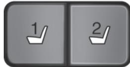
This memory control, located on the driver's door, allows automatic positioning of the driver seat and power mirrors to two programmable positions. You may also have this feature for the steering column and power adjustable foot pedals.
