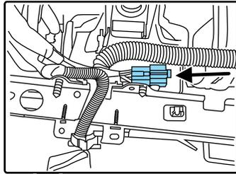
The connector is located under the instrument panel above the brake pedal.
