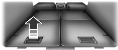
1. Unlatch and lift the seat out of the floor tub by squeezing and pulling up on the handle. Once the seat is at a vertical position, push the seat over, letting it fall onto the latches.
