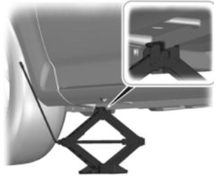
10. Put the jack in the jack notch next to the tire you are changing. Turn the jack handle clockwise until the wheel is completely off the ground.
